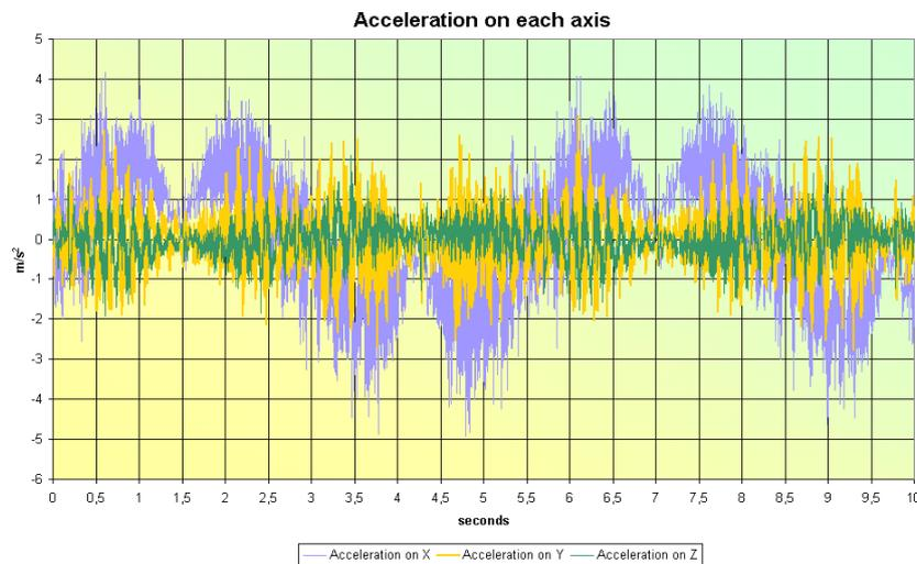
The software *FastTracer* Application is able to download the numeric value pure acceleration data; acceleration data were integrated for obtaining the value in velocity and displacement. Using this computed values it was possible to develop specific conclusions.
