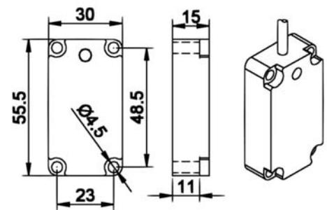
Figure 2: FastTRACER dimensions
