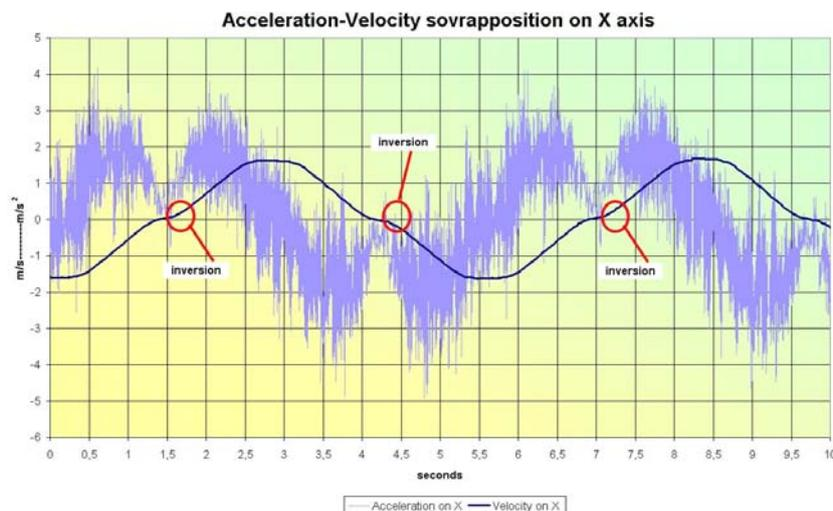
The analysis has been made during the signal acquisition and at the end of the test, had showed the real strains which the Y and Z were subjected to, during the cyclic linear inversion on X axis.
